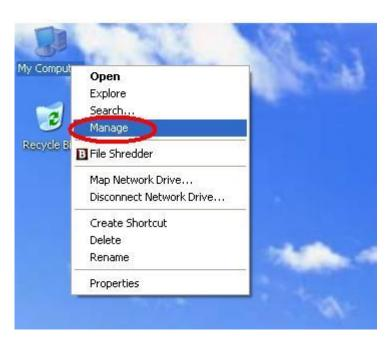
**STEP 6:** Then go to device manager, in that we have to select ports (COM and LPT). There we have to find the COM port which has been selected for USB cable. The same COM has to be select for Flash Magic.
